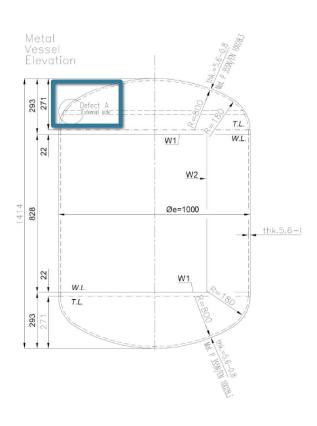
Test 4 - one thickness reduction on the superior end of the tank
