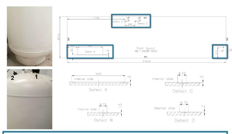
Test 3 – four thickness reductions from 1.0 to 2.0 mm on the shell
