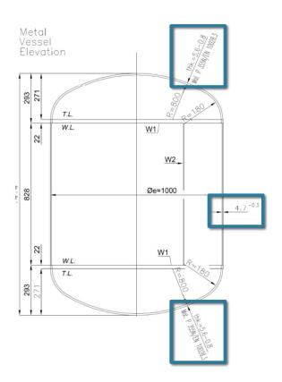
Test 1 - A shell's thickness reduction of 0.9 mm; no artificial defects
