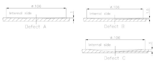
Test 2 - three thickness reductions from 1.0 to 3.0 mm on the shell
